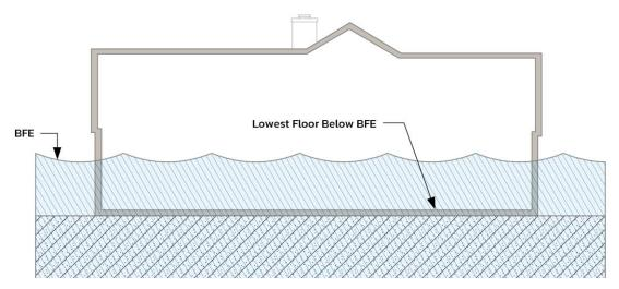
Figure 04.1: Lowest Floor Elevation
