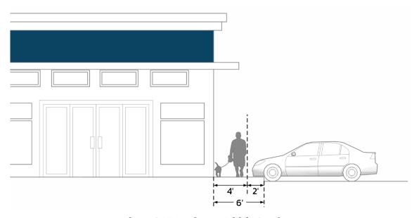
Figure 04.5: Maximum Vehicle Overhang
