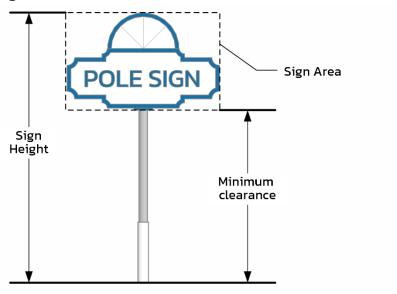
**Figure 05.9: Example Clearance Measurement**
