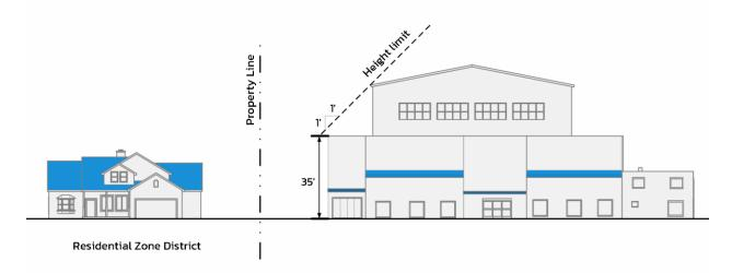
Figure 04.12: Residential Adjacency Horizontal Step Back Requirement
