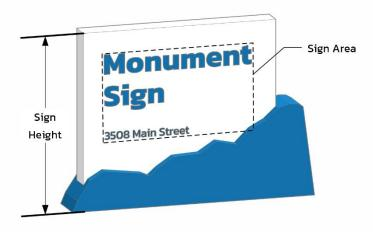
Figure 05.8: Example Sign Height Measurement
